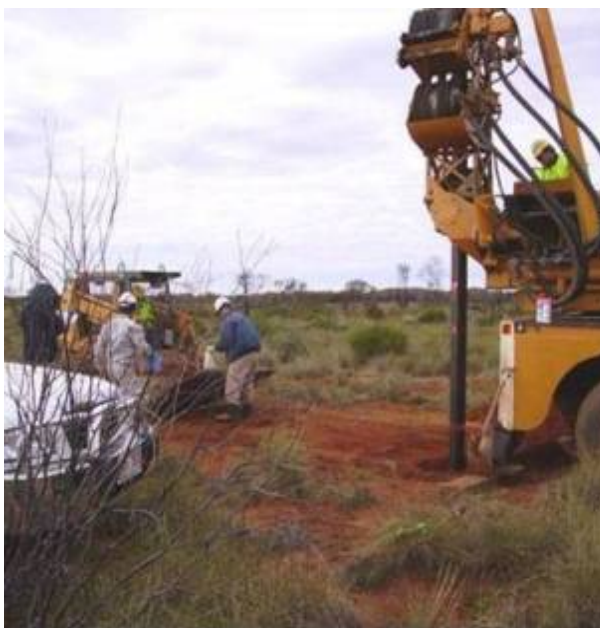
Drilling and sampling above the water table
